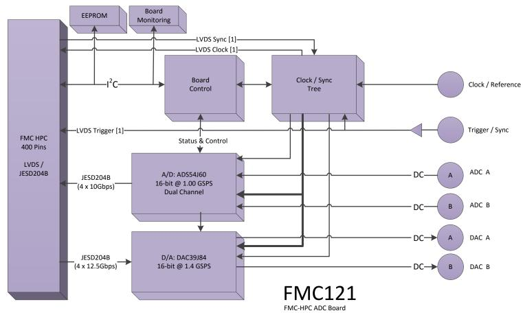
FMC-HPC ADC Board Two Channel 16-Bit A/D up to 1.0 Gsps Two Channel 16-Bit D/A up to 1.4 Gsps
