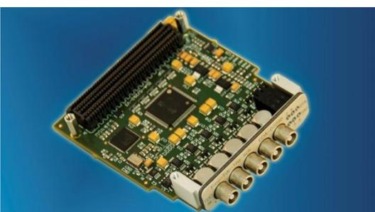
An FPGA Mezzanine Card (FMC) with a Time to Digital Converter chip to perform one-shot sub-nanosecond time interval measurements
