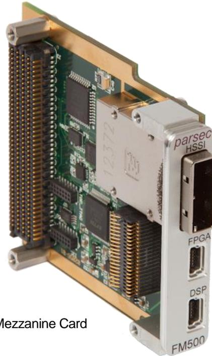
Figure 14: FM500 FPGA Mezzanine Card
