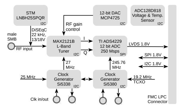
The following figure gives an overview of the components on the FMC satellite receiver board.
