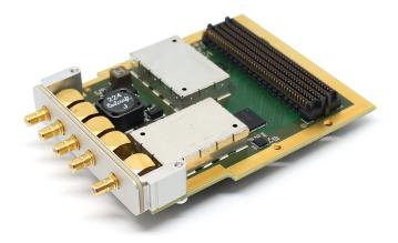
The Creonic L-band RF receiver FMC card allows to receive RF signals between 925 and 2,250 MHz. It is ideally suited for satellite communication with standard satellite dishes since it includes a DiSEqC driver IC for LNB controlling. Due to the low-pin-count (LPC) FMC connector it can be used with all FMC carrier boards that support  $V_{adj} = 1.8V$ .
