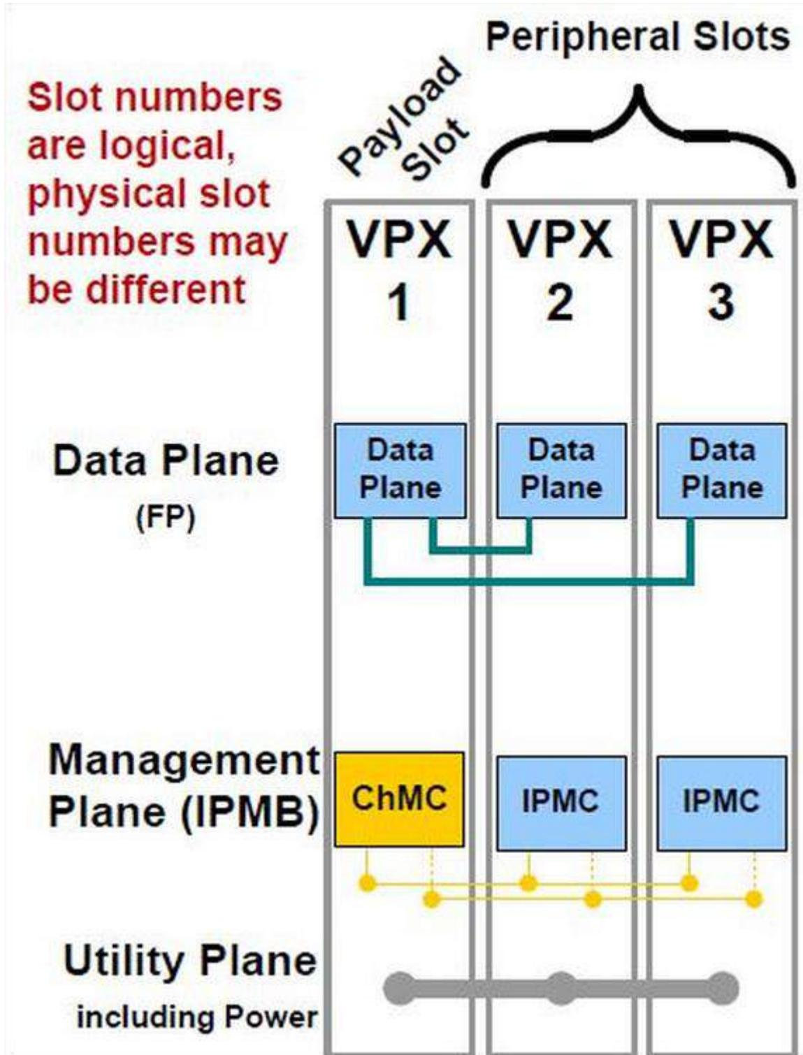
Figure 4: VPX Test Platform Backplane diagram
