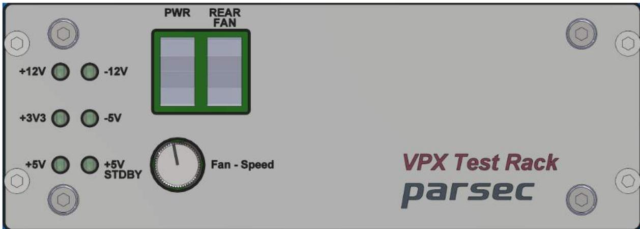
Figure 3: VPX Test Platform Control Panel
