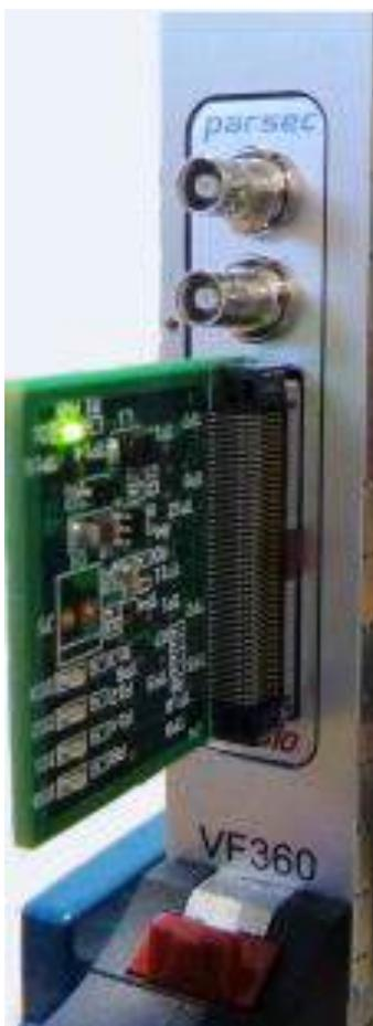
Figure 8: FM510 Loopback board plugged into FM510
