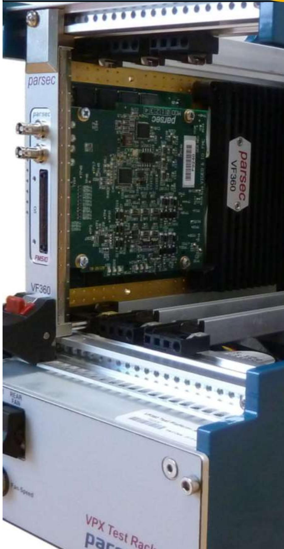
**The VF360 is a 3U OpenVPX module that leverages on Altera Stratix® V FPGA and Texas Instruments KeyStone® Multicore DSP technology to provide an ultra-high bandwidth processing platform, ideally suited for computation and bandwidth intensive applications.**
