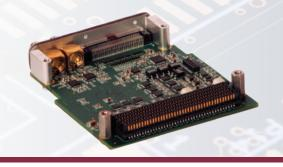
The secondary video and IO interfaces on the high-density connector are accessed by means of an Adaptor Board the connects to the **FM510** front panel.
