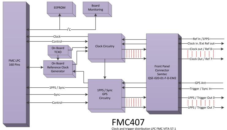
Clock and trigger distribution LPC FMC VITA 57.. Frequencies between 34.375 MHZ and 4.4GHz
